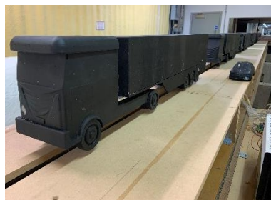
Figure 1. Platoon of five HGV lorries moving above a suspended ground plane with fixed intervehicle spacing of 6 m at full-scale.
